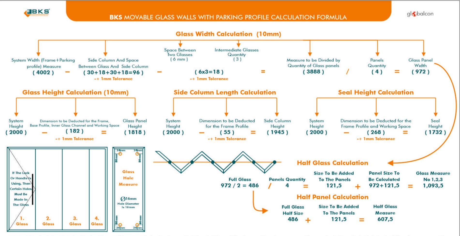
Note: The size to be deducted for the intermediate cover size in glass base calculations is 11 mm. This document has been prepared for our dealer to make technical calculations (measurements).
