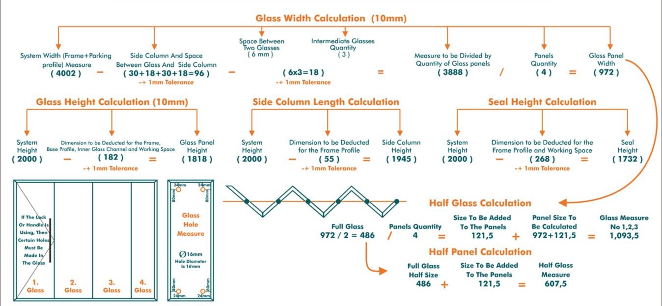
Note: The size to be deducted for the intermediate cover size in glass base calculations is **11 mm**. This document has been prepared for our dealer to make technical calculations (measurements).
