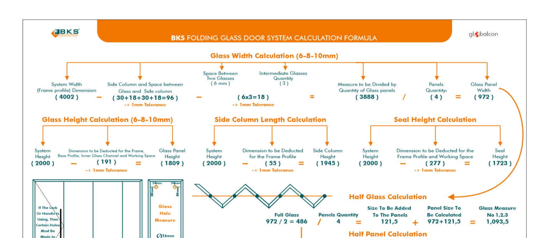
Note: The size to be deducted for the intermediate cover size in glass base calculations is 11 mm. This document has been prepared for our dealer to make technical calculations (measurements). The dimensions specified in the document are prepared as an example Check before production; our company is not responsible for wrong calculations and cuts.
